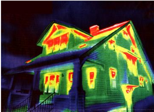
IR image of conductive losses in home
